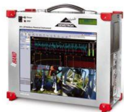
Figure 7: Data Acquisition Unit (DA-121).
