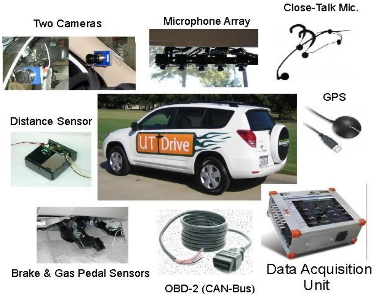
Figure 9: UTDrive's data-collection vehicle and its components.
