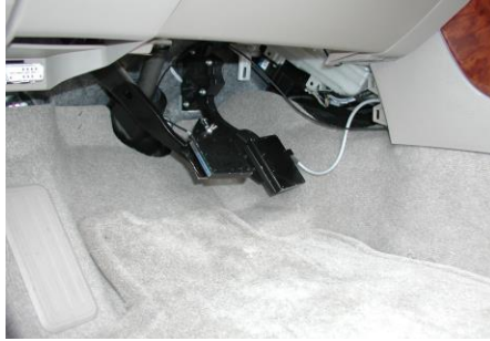
Figure 3: Brake and Gas pedal pressure transducers.
