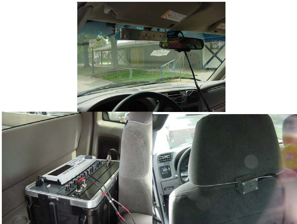
Figure 7: Chevy S10 Extended Cab Pickup Truck: Data Collection Setup: (a) Microphone array position, (b) digital data recorder position, (c) Reference microphone and positioning behind driver seat (note: photo taken through rear window towards driver's seat).
