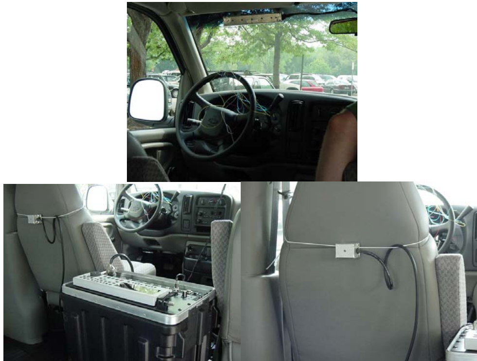
Figure 6: Chevy Express Van: Data Collection Setup: Microphone array position, digital data recorder position, Reference microphone and positioning behind driver seat.
