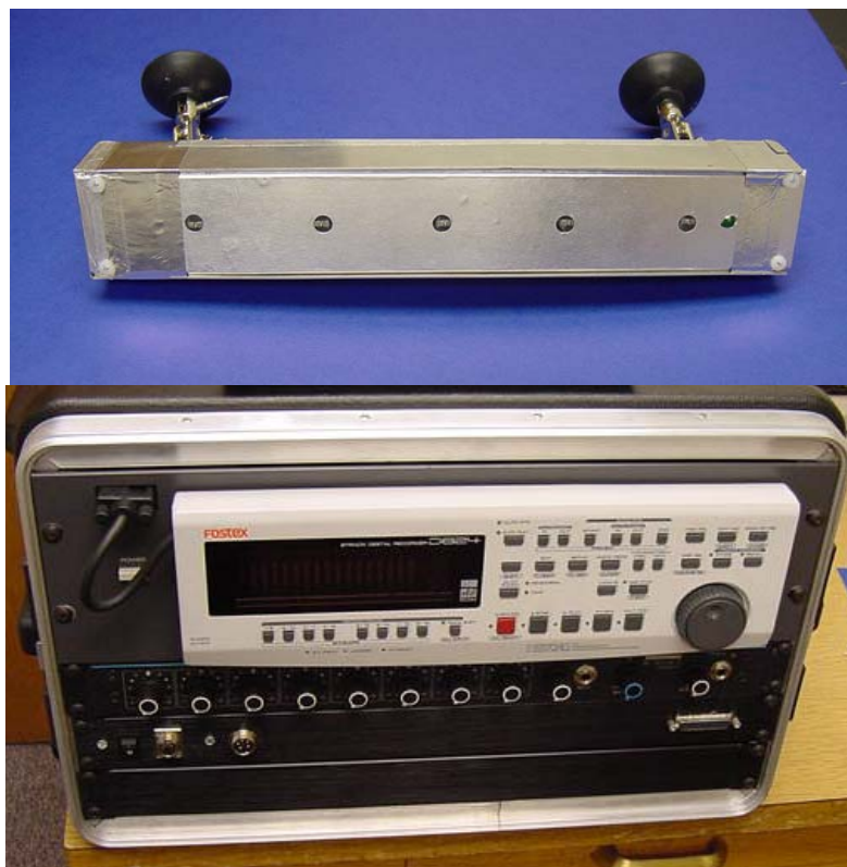
Figure 2: CSLR Microphone array (early proto-type) and constructed 8-channel digital recorder system.
