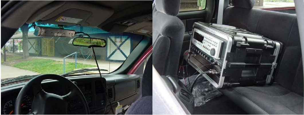
Figure 8: Chevy Silverado Pickup Truck : Data Collection Setup: Microphone array position, digital data recorder position, Reference microphone and positioning behind driver seat (note: photo taken through rear window towards driver's seat).
