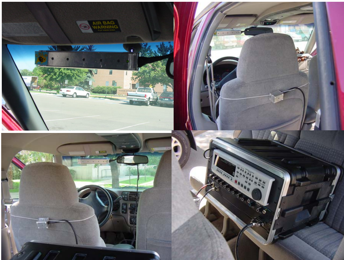
Figure 9: Chevy SUV Blazer : Data Collection Setup: Microphone array position, digital data recorder position, Reference microphone and positioning behind driver seat.
